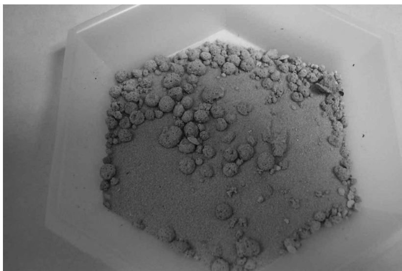
Figure 3. Bed material from Feed #3 Run #3 contained large diameter spherical particles that appear to be pieces of deposits that have broken off and been ground into spheres.
